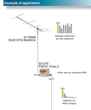
to the multiband amplifier band 3 or VHF input
