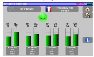
If the device is not synchronized across all four channels, the quality indicator is red.
