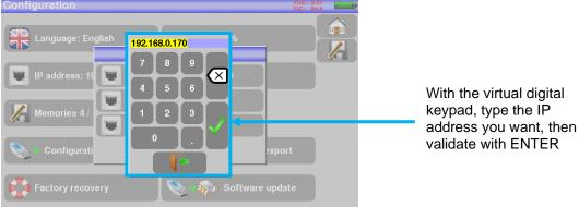
The PC software in communication with the appliance must have the same IP address as the appliance, just like in the example below:
