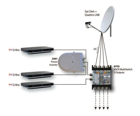
The powersupply is designed to power the dSCR output, in case the STB can not provide enough DC power. See diagram above for a typical installation.
