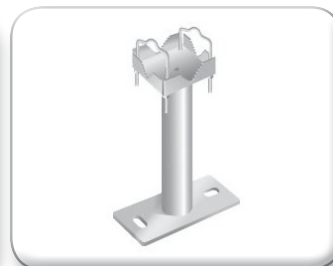
Zanca attacco ganancia 15 cm Art. 07-483 Palo Ø 30÷70 mm Piastra 200x70x4 mm
